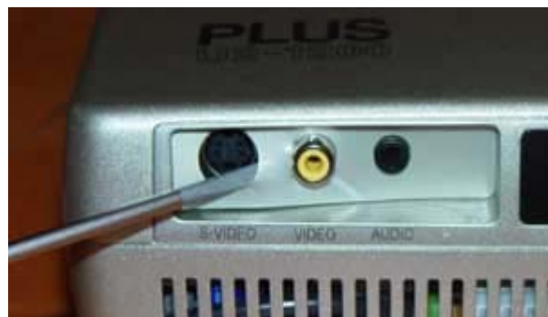
Figure 2: Use a Flat head screwdriver to help pry the sticker off
