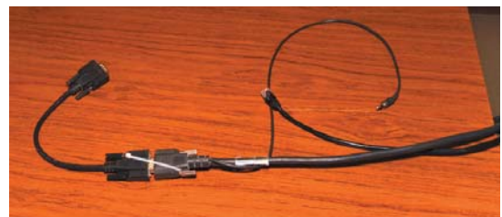
Cable fan-outs make repairs easy.
