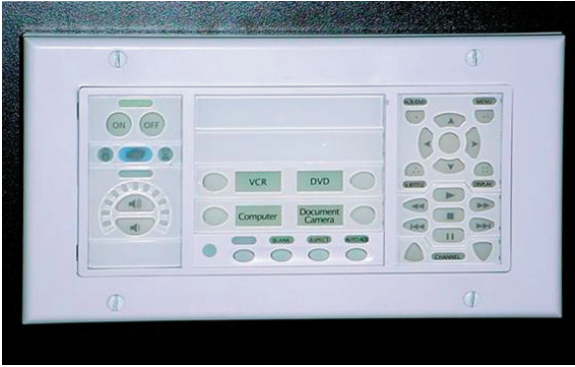
SP Controls' PixiePro panel replaces remote controls for the projector, DVD player and other equipment, making AV control simple.
