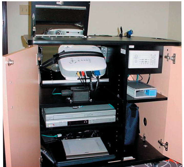
Inside view of an AV cart. The projector throws a reverse image onto a mirror, which bounces to the classroom screen. The SP Controls PixiePro panel, which controls all of the equipment in the cart, is to the right of the projector.
